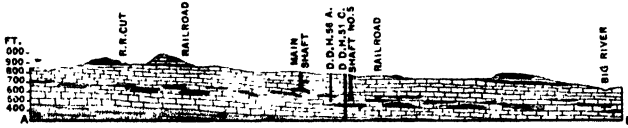
FIG. 123.—Section at Bonne Terre, Mo., showing ore disseminated through limestone.
